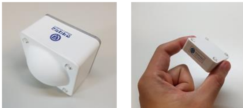
Figure 36 Illustration of lens antennas with planar and curved shapes
