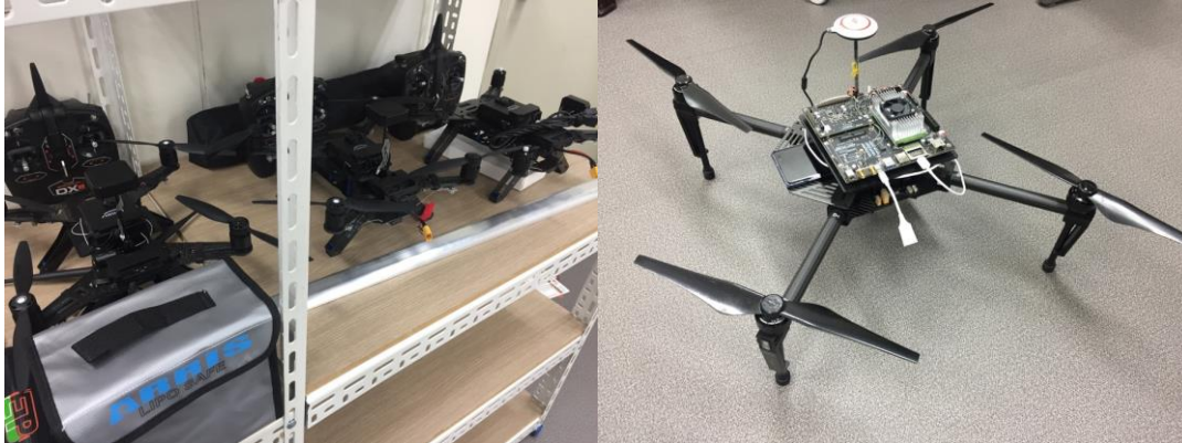
Figure 15 Intel Aero RTF drone fleet members (left) and DJI Matrice 100 drone (right) at YU
