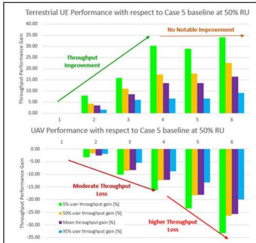
Figure 5-3: Uplink terrestrial UE and UAV throughput results with different P_0 values for UAVs and terrestrial UEs considering 50% resource utilization. Baseline scheme is Combination-1 in Table 5-1 [42].
