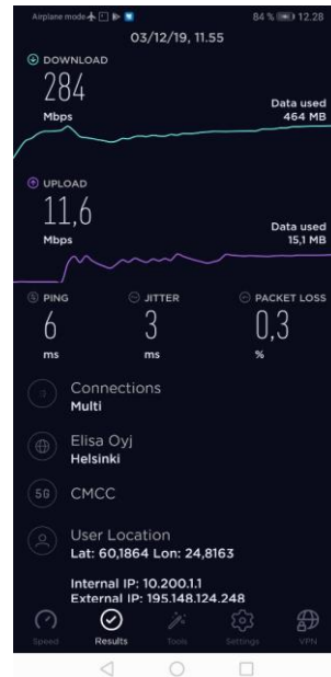
Figure 15. Speedtest showing the latency and throughput measured in the 5G capable mobile device.
