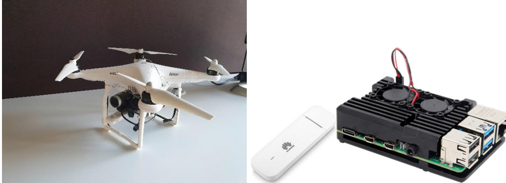
Figure 4: UAV with rPI, LTE USB dongle and video camera.
