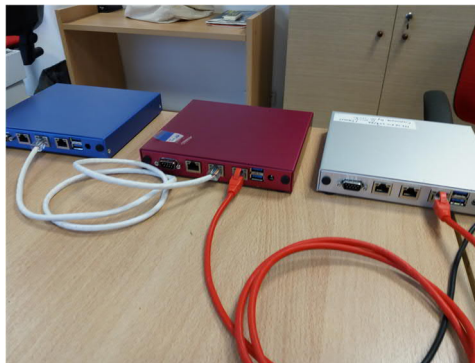
Figure 9: Linux servers with packet core in red and SDN switches in blue and gray boxes.
