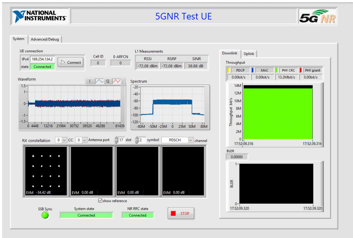
Figure 16: 5G NR Test UE in connected mode reaching PDSCH throughput of 13.2 Mbit/s
