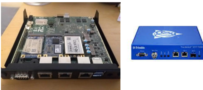
Figure 6: Linux server running 4G/5G core and Trimble Grand Master.
