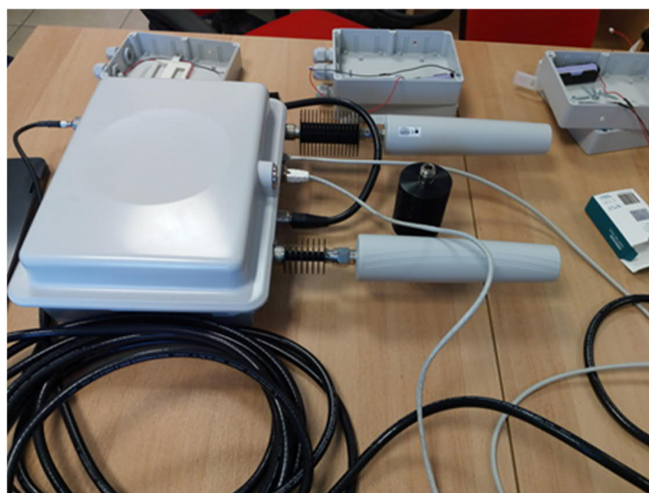
Figure 10: Commercial eNB with NB-IOT configuration in 1.8GHz
