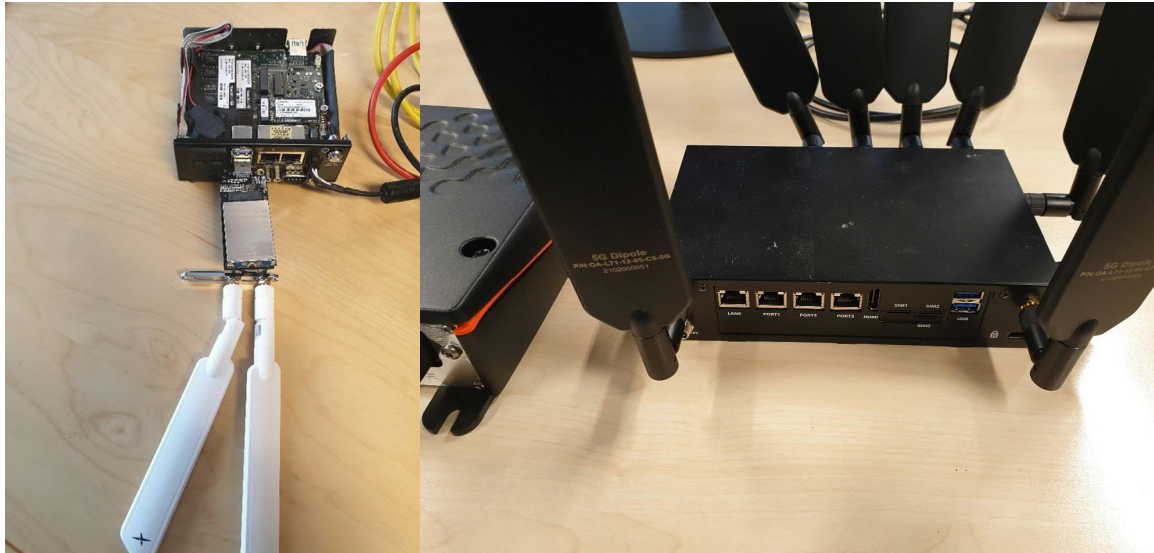
Figure 10. Devices for the Interoperability testing 5GC and Aalto gNB SA.
